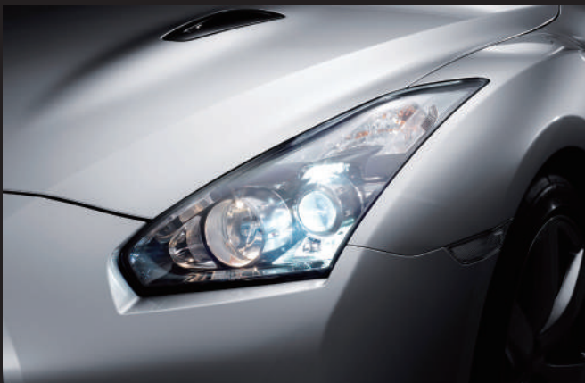
Equipped with newly developed super wide-beam headlamps that include three additional auxiliary reflectors, enabling wider illumination.
